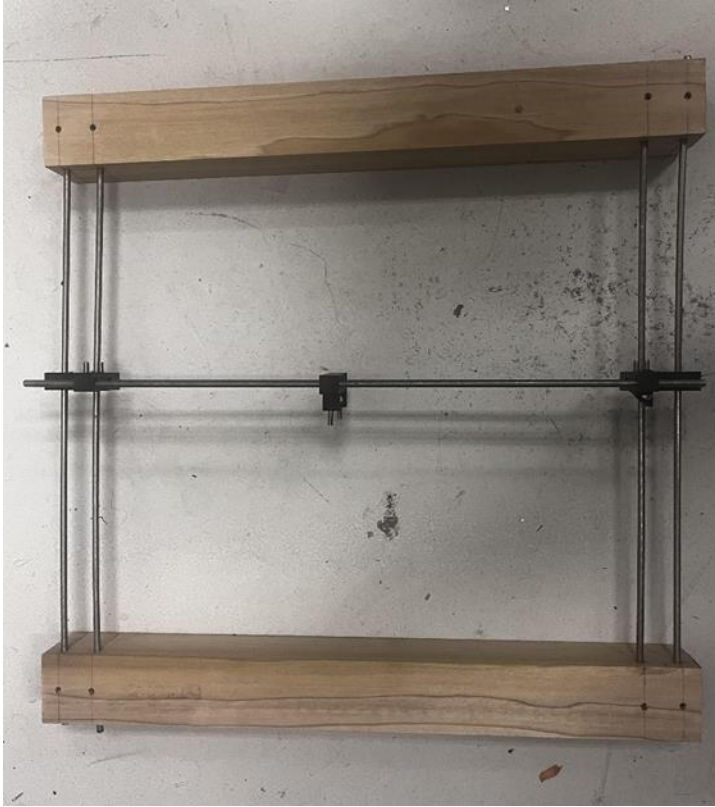
Figure 29: Rough gantry prototype used for demonstration
