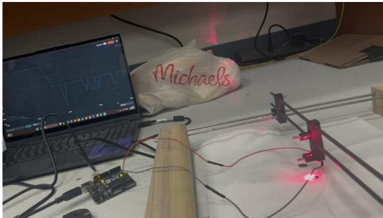
Figure 45: The carriage was just moved onto a black spot on cotton fabric. Photodiode readings on the graph on the left show significantly reduced back-reflections.
